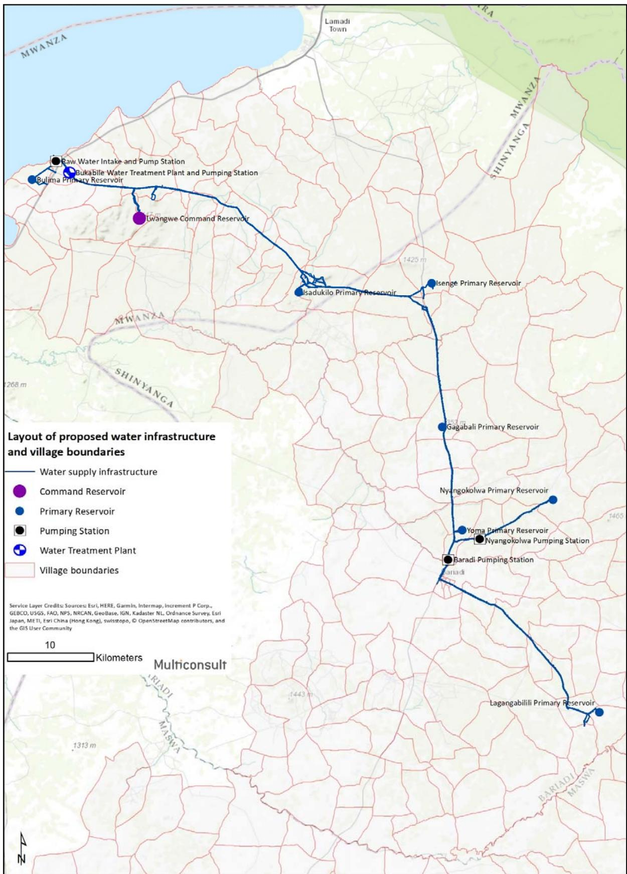
Figure 2: Routing of water main for Phase 1 with new locations of water treatment plant and reservoirs.
